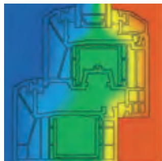
Thermal insulation - The thermal image shows the optimised distribution of isotherms
